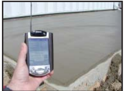
Handheld PC communicating with a buried tag
