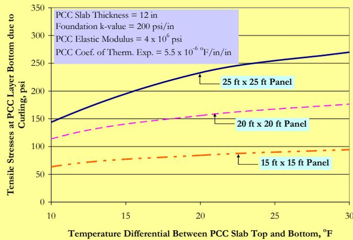
The impact of slab aspect ratio on PCC curling stresses is illustrated below as a function of the foundation  $k$ -value. Clearly panels with higher aspect ratios lead to higher curling stresses. Further, high aspect ratios lead to critical stress development over a wider portion of the slab span (not shown here), thereby increasing the probability of cracking.
