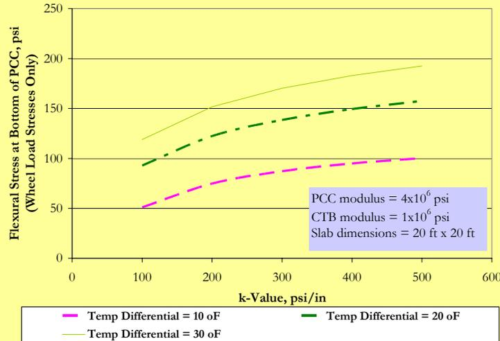
Higher curling stresses can lead to higher combined stresses (load plus curl) in pavements. Therefore, while a thicker base can lower stresses due to wheel loads, this advantage is negated to a degree by an increase in the curling stresses.
