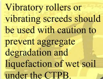
Vibratory rollers or vibrating screeds should be used with caution to prevent aggregate degradation and liquefaction of wet soil under the CTPB.
