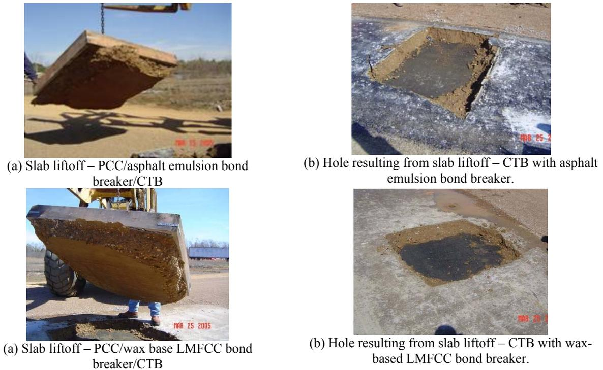
Figure 2-5. Slab liftoff tests with conventional curing compounds.
