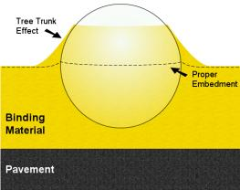
FIGURE 6-65. WICKING MATERIAL OVER BEAD.
