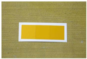
FIGURE 6-73. YELLOW COLOR CHIP COMPARED TO YELLOW MARKING.
