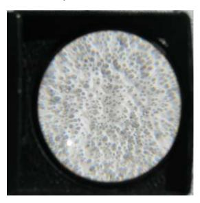
FIGURE 3-5. GOOD TYPE I BEAD DISTRIBUTION; READINGS AVERAGED 300 mcd/m²/lux.
