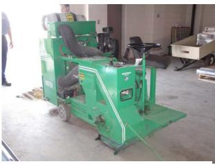
FIGURE 5-13. SHOTBLASTER WITH A 10-INCH CUT.
