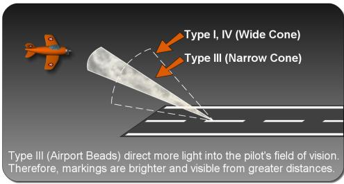
FIGURE 3-6. DEMONSTRATES THE GREATER RETURN OF LIGHT FROM THE 1.9 IOR (TYPE III GLASS BEADS) WHEN COMPARED TO THE 1.5 IOR (TYPE I OR TYPE IV GLASS BEADS).
