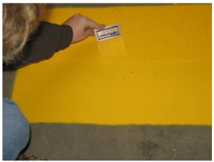
FIGURE 6-62. USE OF WET FILM GAUGE.
