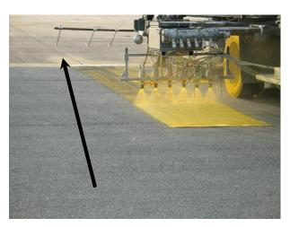
FIGURE 6-54. MECHANICAL POINTER.
