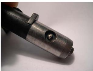
FIGURE 6-18. AIRLESS SPRAY TIP.
