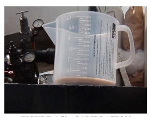
FIGURE 6-59. CALIBRATION BUCKET FOR GLASS BEADS.
