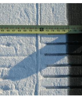
FIGURE 2-3. MARKING DIMENSION IS OUT OF TOLERANCE.
