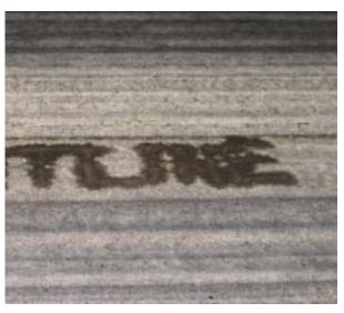
FIGURE 4-31. RUST REMOVER DAMAGED GLASS BEADS, MAKING THEM INEFFECTIVE.
