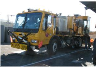
FIGURE 6-24. TRUCK-MOUNTED AIRPORT STRIPING EQUIPMENT.
