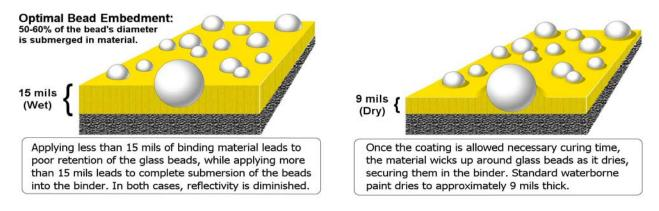
FIGURE 3-12. GLASS BEAD EMBEDMENT IN BOTH WET AND DRY PAINT FILM.
